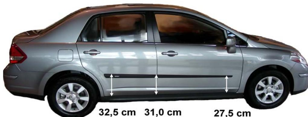
This Side Moulding Kit is designed to be fitted according to the measurements given on the photo.
